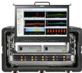
GaGe wideband receivers feature up to 3 software selectable IF bandwidths, from 10 MHz to 160 MHz. The RF signal tuning covers 50 MHz to 27 GHz to provide unparalleled real-time signal recording and analysis capability ideally suited for use with the RazorMax digitizer's 16-bit resolution and 500 MS/s sample rate.
