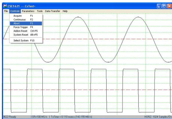
The included and more advanced GaGeScope Lite Edition is a solutions oriented PC oscilloscope application that allows users to quickly and easily control the digitizers without having to write a single line of code. Data can be displayed, analyzed, printed and saved with an easy-to-use Windows-based user interface.
