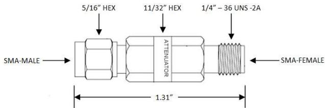
The table below lists available inline attenuators with their Attenuations in dB, Scaling Factor, and Effective Input Range that results when applied to the single fixed lower  $\pm 240$  millivolts input range RazorMax Express models.
