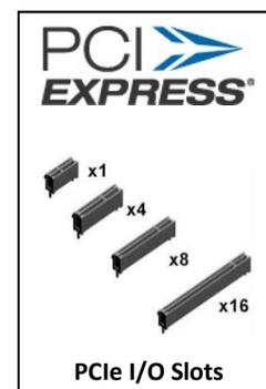
The RazorMax Express is fully backwards compatible with previous PCIe Gen2 and Gen1 based slots. It is also possible to operate
