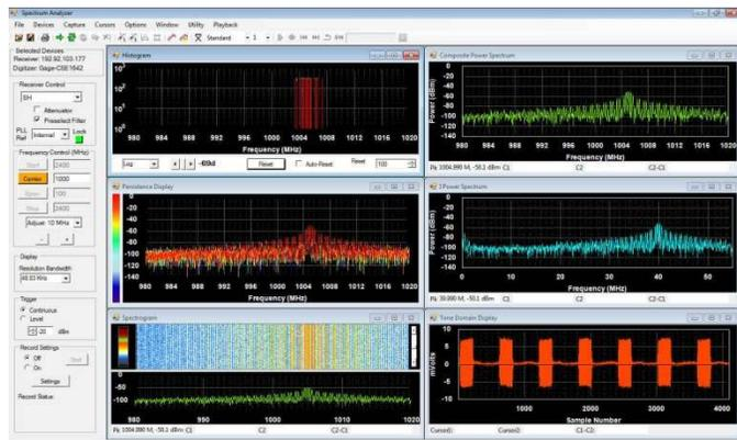
SpectraScopERT features real-time FFT power spectrums (with peak hold and persistence), spectrograms, histograms, and time domain displays while recording, and upon recording playback.
