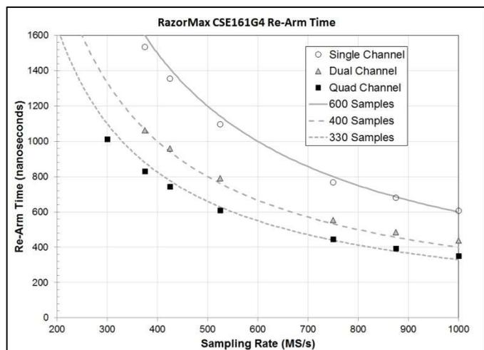
**Figure: Re-Arm Times at 1 GS/s Sampling Rate**
