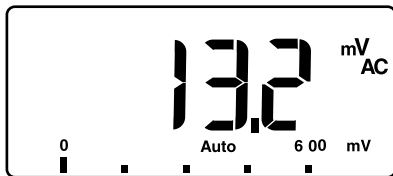
Figure 1. Residual Voltage Reading
