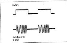
Fig. 7-12 A two-tone burst with its sync-pulse.
