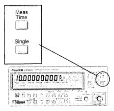
MEAS TIME The measuring time is preset to 200ms. This gives nine digits on the display, and four measurements each second.
