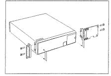
Fasten the PM6685 or PM6685R in the rack via screws in the four rack mounting holes
