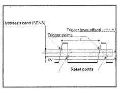
Fig. 6-1 Frequency is measured as the inverse of the time between the one trigger point and the next.
