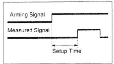
Fig. 7-6 Time from active external control edge before the measurement is armed: E channel . < 5 ns
