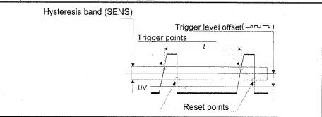
Fig. 5-2 Parameters controlled by SENS and Waveform keys.
