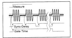
**Fig. 6-8** Measuring Burst Pulse Repetition Frequency.
