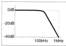
Fig. 5-4 Characteristics of LP filter.
