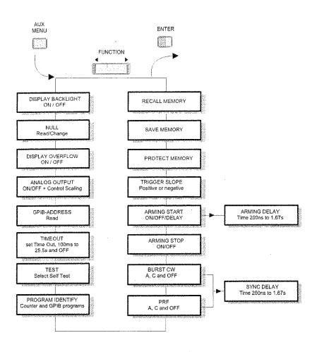
Fig. 9-1 You will enter the AUX MENU at the same selection as you used the previous time, except after power on when you enter the menu at RECALL. To recall the last setting before power off, recall memory 0.
