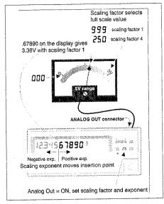
Fig. 9-2 The analog output function.
