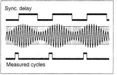
Fig. 6-12 Effects of different sensitivity when measuring the CW Frequency of an AM signal.
