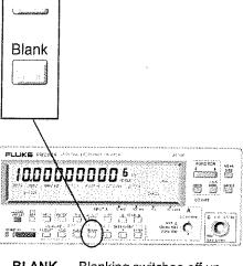
BLANK DIGITS Blanking switches off unnecessary digits on the display. Press **BLANK DIGIT** once for each digit you want blanked.
