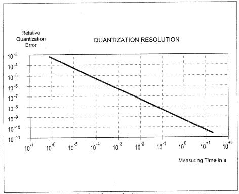
Fig. 7-2 Resolution as a function of measuring time.
