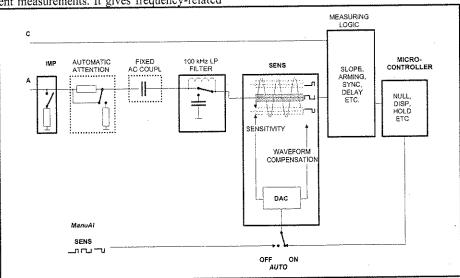
Fig. 5-1 PM6685 Signal Conditioning Block Diagram.
