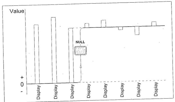
Press the **NULL** key to store the current result as a constant, and switch on the nulling function. The counter will now show the results as a deviation from the stored constant.
