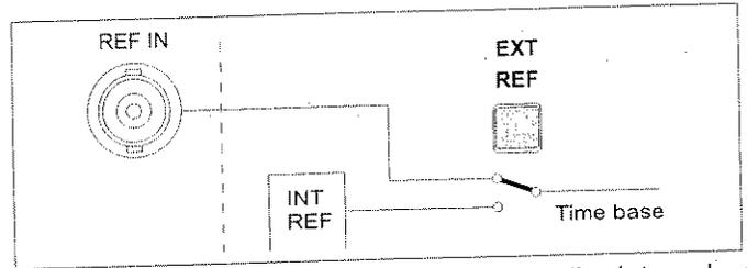
Press the **EXT REF** key to toggle between the internal or external 10 MHz time-base. Since no reference signal is connected the display will show 0.
