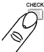
The **CHECK** key enables a self-test of the measuring functions. Press the **CHECK** key to connect internally the 10 MHz reference signal to the logic circuit. Press the **FUNCTION** rocker key to scroll through all measuring functions.
