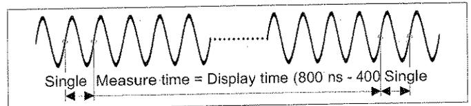
Turn on **SINGLE**. The result is now from a single measurement cycle, and the "measuring time" becomes display time (time between measurements). This gives fast measurements with low resolution.
