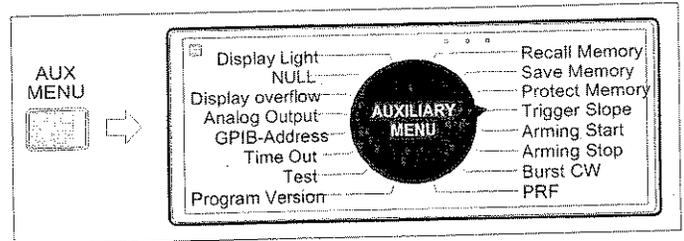
Regard the AUX MENU as a rotary switch. Press the **AUX MENU** key and then use the **FUNCTION** rocker to "turn" the rotary switch. When the display shows the function you want, confirm your selection by pressing **ENTER** key. To escape without selecting any auxiliary function, press the **MEAS RESTART** key.
