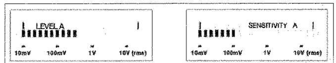
The bar graph scale has two functions: It shows the input level when AUTO is on, and the sensitivity setting when AUTO is turned off.
