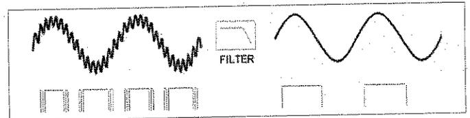
Press the **FILTER** key to toggle the built-in 100 kHz LP filter. The filter segment is on when the filter is being used.
