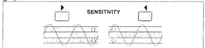
Turn on **AUTO**, and then turn it off again by pressing one of the **SENS** keys. This way you freeze the current waveform selection and sensitivity selected by **AUTO**. Pressing **SENS** again will increase/decrease the sensitivity around the frozen waveform compensation.
