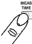
The measuring time decides the resolution in the measurement. Increasing the measuring time gives more digits. Press the **MEAS TIME** key and use the **FUNCTION** rocker key to change the measuring time in steps of 1-2-5 as coarse adjustment. Press the **MEAS TIME** key again to return to measuring.
