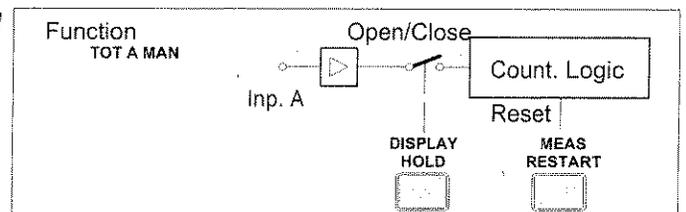
This function lets you totalize (count) the number of trigger events on channel A. Use the **DISPL HOLD** key to start and stop totalization, and the **MEAS RESTART** key to reset the displayed result.
