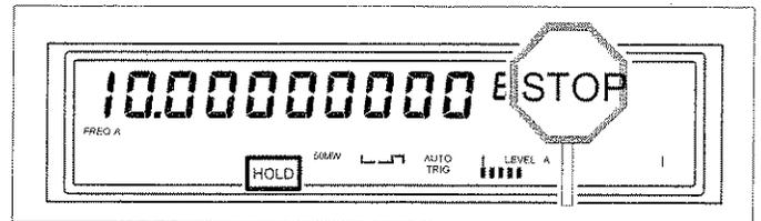
Press the **DISPLAY HOLD** key to hold the current readout on the display. Press again to continue to measure. When **DISPLAY HOLD** is active, a new measurement is made each time you press **RESTART**.
