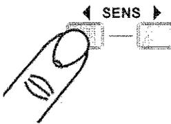
Use the **SENS** keys to adjust the input sensitivity. You can read the current sensitivity setting on the bar graph.
