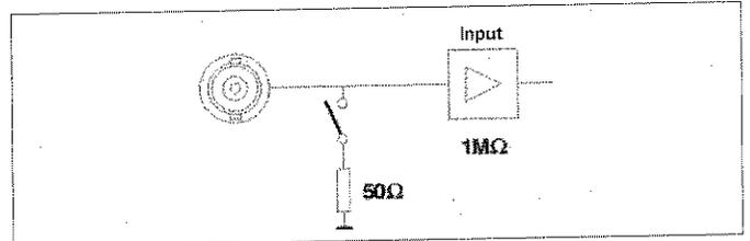
Press the **50Ω** key to toggle between **50Ω** and **1MΩ** termination on input A. Your selection is shown on the display. If the counter refuses to switch to **50Ω**, the input signal is above the safe limit of 12 Vrms.
