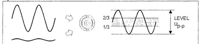
You'll soon find that it's much easier, and more accurate to measure with the AUTO function on, than to do manual settings. There are just a few exceptions that needs manual settings - AM-modulated signals, extremely noisy signals, non-repetitive signals, and signals with frequencies below 50 Hz.
