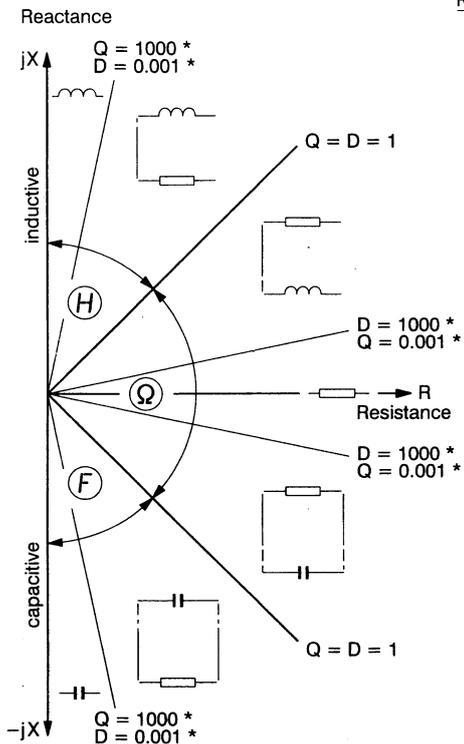
\* For test signal voltages  $\leq 0.25$  V, the decision criterion is  $Q = 200$ ,  $D = 0.05$ , or  $Q = 0.05$ ,  $D = 200$
