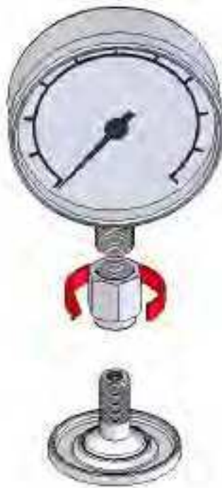
Figure 2-1. Screw on Gauge Adapter
