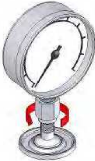
Figure 2-2. Connect Assembly to Test Port
