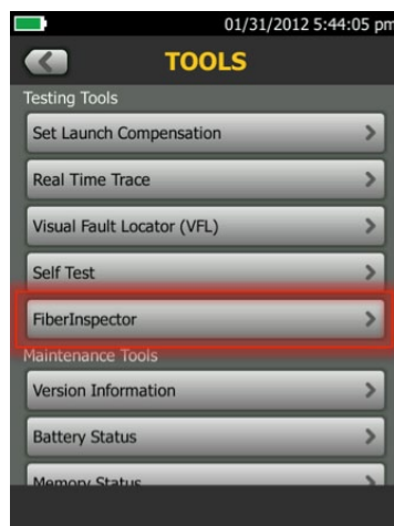
Figure 25 - FiberInspector set up from Tools menu
