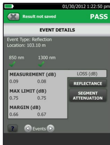
Figure 13 - OptiFiber Pro EventMap™ example, by tapping on bubble to drill in for more information
