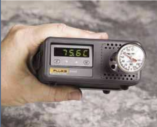
Temperature sensor calibration is easy with a handheld dry-well.
