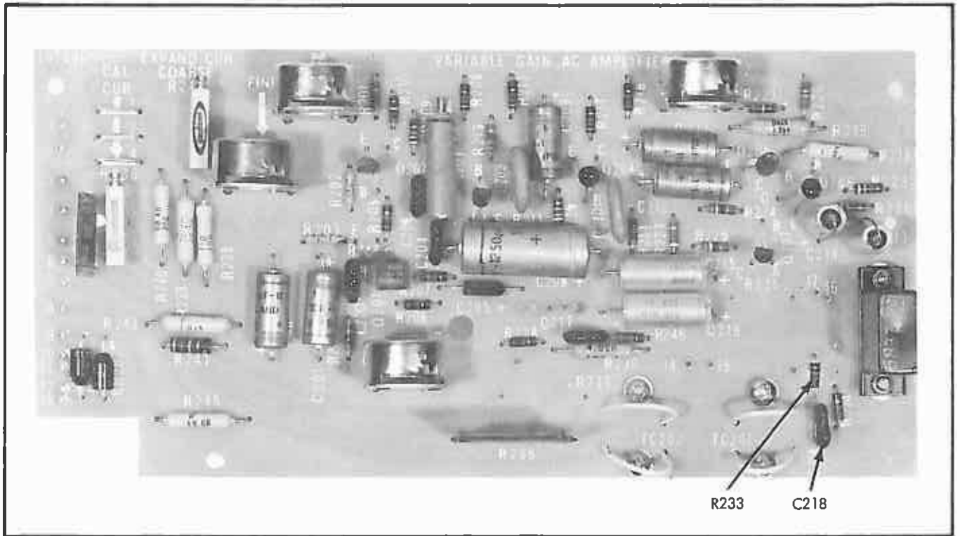
Figure 4-25. LOCATION OF COMPENSATING NETWORK COMPONENTS
