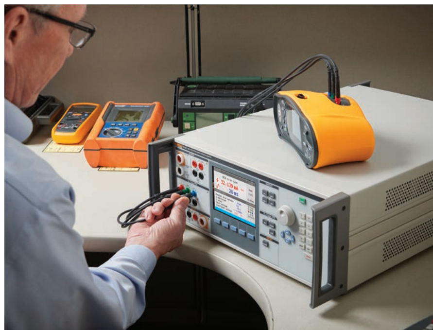
Each 5322A comes with an external R-Multiplier to source resistances of up to 10 TΩ for testing insulation testers.
