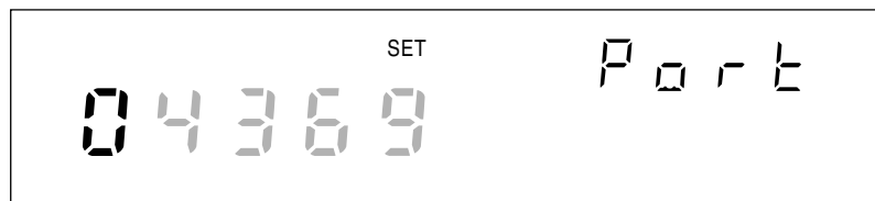
Socket Port display for setting the first digit (for the example 0 4369)
