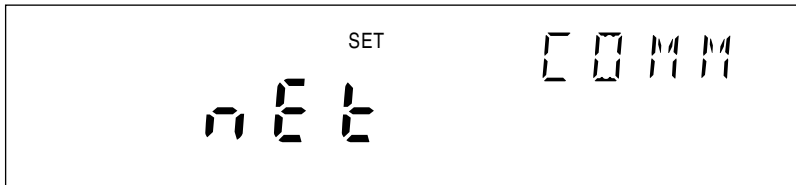
Communications display for setting the network type
