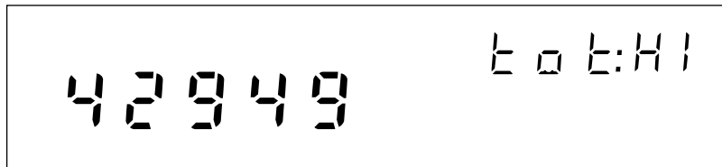
Totalizer status display for the high digits (for the example 42949 67295)
