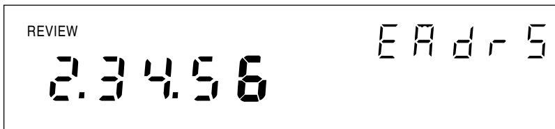
Ethernet address display for viewing byte 5 (for the example 00-80-40-12-34- 5 6)
