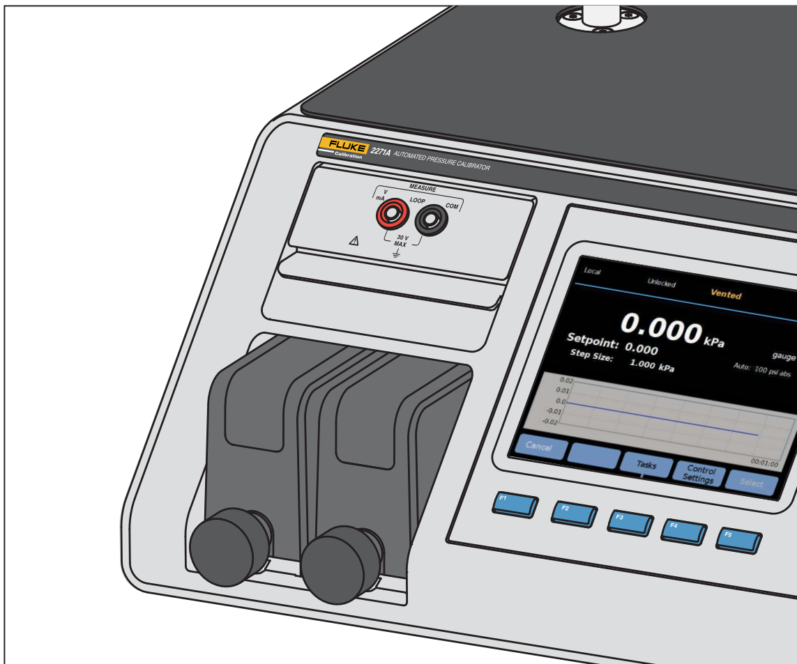
Figure 3. Installed EMM and PMM Modules
