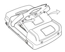
Figure 49. Removing the Battery Cover
