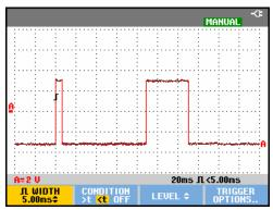
Figure 33. Triggering on Narrow Glitches
