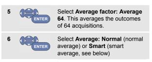
You can use the average functions to suppress random or uncorrelated noise in the waveform without loss of bandwidth. Waveform samples with and without smoothing are shown in Figure 9.
