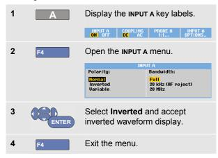
For example, a negative-going waveform is displayed as positive-going waveform which may provide a more meaningful view. An inverted display is identified by an inversed trace identifier ( ) at the right of the waveform, and in the status line below the waveform.
