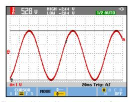
Figure 25. Voltage Measurement with Cursors
