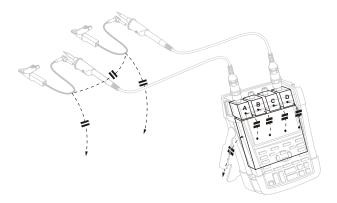
Figure 40. Parasitic capacitance between probes, instrument and environment
