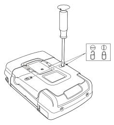
Figure 48. Unlocking the Battery Cover
