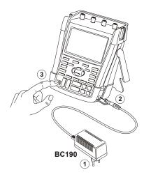
Figure 2. Powering the Test Tool
