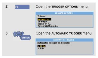
If the frequency range of the automatic triggering is set to > 15 Hz, the Connect-and-View™ function responds more quickly. The response is quicker because the test tool is instructed not to analyze low frequency signal components. However, when you measure frequencies lower than 15 Hz, the test tool must be instructed to analyze low frequency components for automatic triggering:
