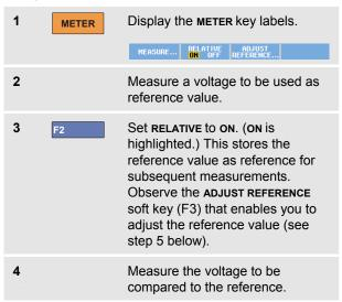
Now the large reading is the actual input value minus the stored reference value. The actual input value is displayed below the large reading (ACTUAL: xxxx), see Figure 13.
