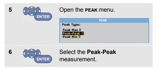
Figure 8 shows an example of the screen with two readings. The character size will be reduced when more then two readings are on.
