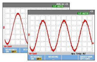
Figure 9. Smoothing a Waveform
