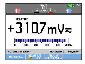
Figure 18. Making a Relative Measurement
