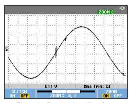
Figure 24. Zooming in a Waveform
