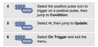
The test tool is now prepared to trigger on pulses that are more than a selectable time in duration. Observe that the trigger menu at the bottom of the screen has been adapted to set the pulse condition:
