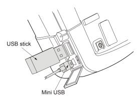
Figure 35. Test Tool USB Connections
