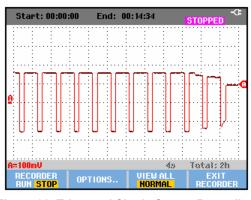
Figure 22. Triggered Single Sweep Recording
