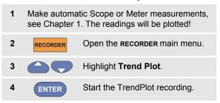
The test tool continuously records the digital readings of the measurements and displays these as a graph. The TrendPlot graph rolls from right to left like a paper chart recorder.
