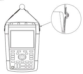
Figure 46. Fixing the Hangstrap
