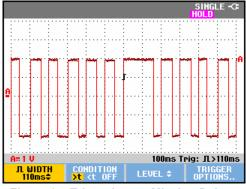
Figure 34. Triggering on Missing Pulses
