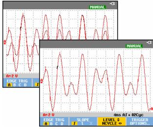
Figure 31. N-Cycle triggering
