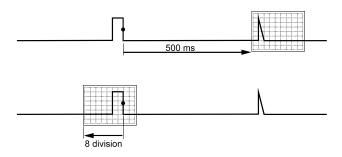
Figure 29. Trigger Delay or Pre-trigger View
