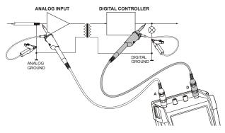
Figure 43. Correct connection of reference leads
