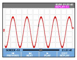
Figure 23. Replaying a Waveform
