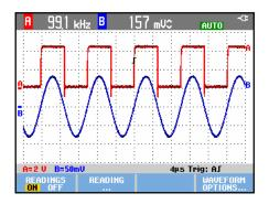
Figure 8. Hz and V peak-peak as Scope Readings
