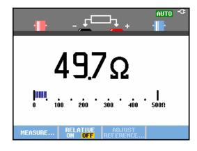
Figure 15. Resistor Value Readings
