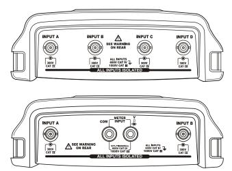
Figure 5. Measurement Connections
