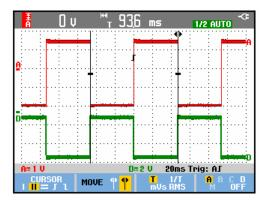
Figure 26. Time Measurement with Cursors
