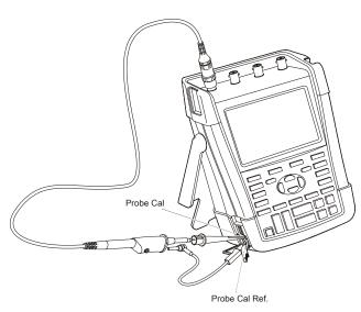
Figure 51. Adjusting Voltage Probes
