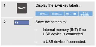
The file is saved using a fixed name (IMAGE) and a serial number, for example IMAGE004.bmp.
