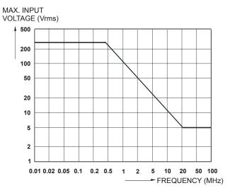
Figure 52. Max. Input Voltage vs. Frequency
