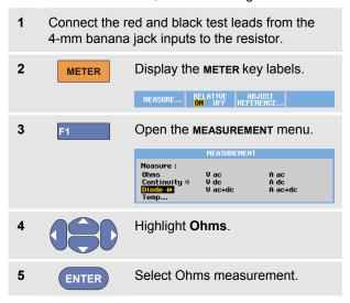
The resistor value is displayed in ohms. Observe also that the bargraph is displayed. (See Figure 15.)
