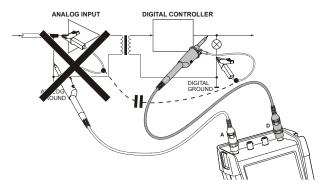
Figure 44. Wrong connection of reference leads
