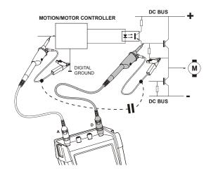
Figure 42. Parasitic capacitance between analog and digital reference
