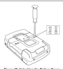
Figure 47. Unlocking the Battery Cover
