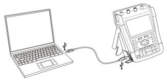
Figure 36. Connecting a Computer
