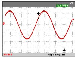
Figure 28. Screen with all Trigger Information
