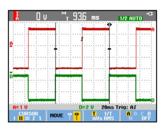
Figure 26. Time Measurement with Cursors
