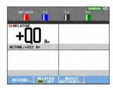
Figure 13. Making a Relative Measurement
