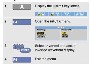
For example, a negative-going waveform is displayed as positive-going waveform which may provide a more meaningful view. An inverted display is identified by an inversed waveform identifier ( **H** ) at the right of the waveform, and in the status line below the waveform.
