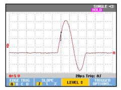
Figure 30. Making a Single Shot Measurement
