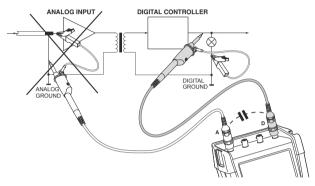
Figure 43. Wrong connection of reference leads
