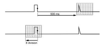
Figure 29. Trigger Delay or Pre-trigger View
