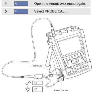
Figure 50. Adjusting Voltage Probes
