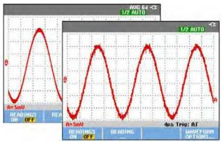
Figure 9. Smoothing a Waveform
