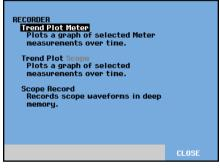
Figure 19. Recorder Main Menu Trendplot Meter is only present in models 190-xx2.
