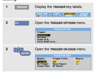
When Free Run is selected, the test tool updates the screen even if there are no triggers. A waveform always appears on the screen.
