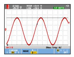
Figure 25. Voltage Measurement with Cursors
