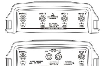
Figure 5. Measurement Connections
