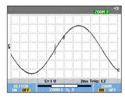
Figure 24. Zooming in a Waveform
