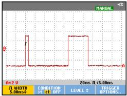
Figure 33. Triggering on Narrow Glitches
