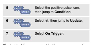
The test tool is now prepared to trigger on narrow pulses only. Observe that the trigger key labels at the bottom of the screen have been adapted to set the pulse conditions:
