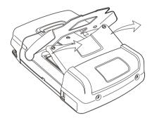
Figure 48. Removing the Battery Cover
