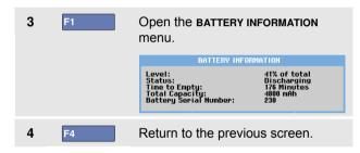
'Level' indicates the available battery capacity as a percentage of the present maximum battery capacity.
