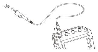
Figure 37. HF Voltage Probe Connection Using **Ground Spring**
