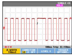
Figure 34. Triggering on Missing Pulses
