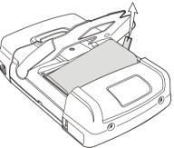
Figure 49. Removing the Battery
