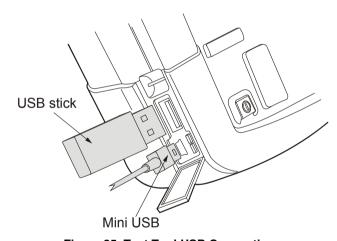
Figure 35. Test Tool USB Connections
