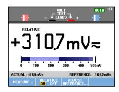
Figure 18. Making a Relative Measurement
