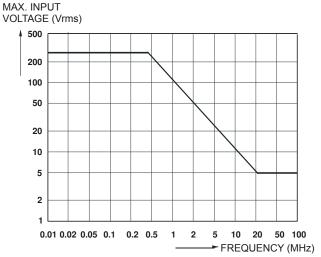
Figure 51. Max. Input Voltage vs. Frequency
