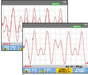
Figure 31. N-Cycle triggering
