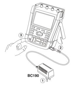
Figure 2. Powering the Test Tool
