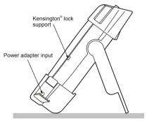
Figure 44. Using the Tilt Stand
