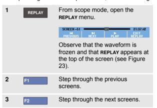
Observe that the bottom of the waveform area displays the replay bar with a screen number and related time stamp:
