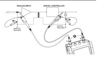
Figure 42. Correct connection of reference leads
