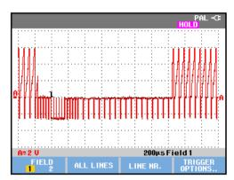
Figure 32. Measuring Interlaced Video Signals
