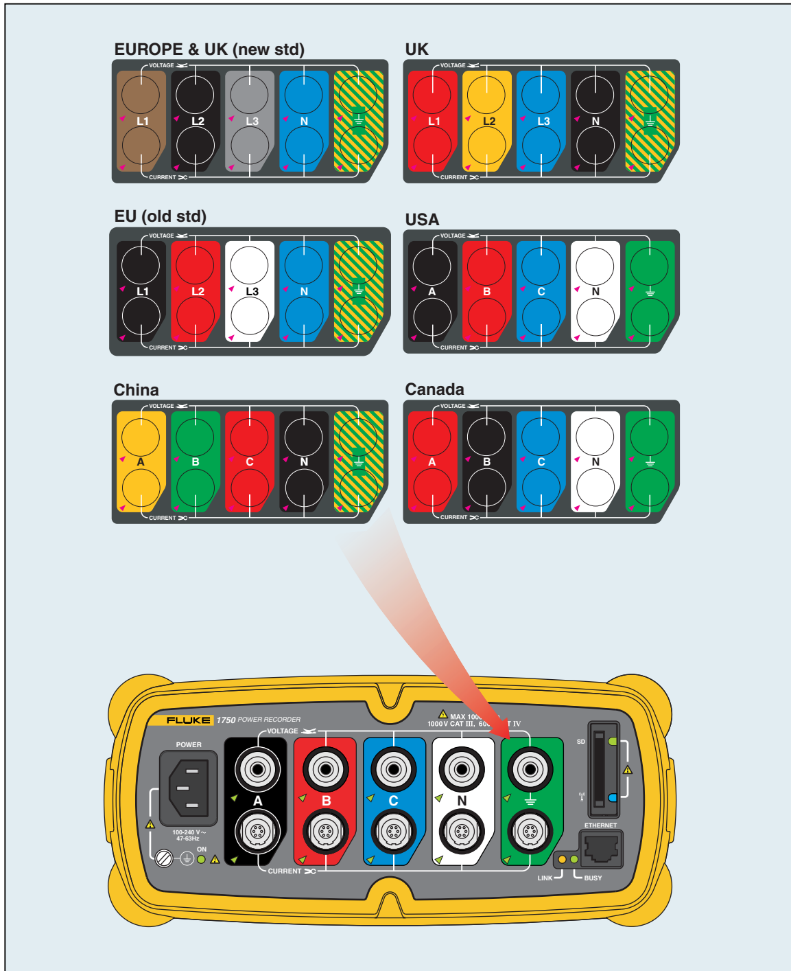
Figure 2. Applying the Front Panel Decal
