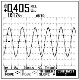
Figure 1-9. Making a Relative Measurement
