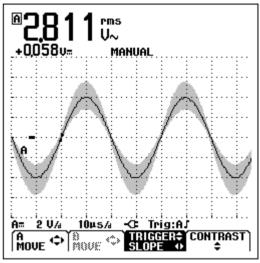
Figure 1-12. Displaying the Envelope of a Waveform
