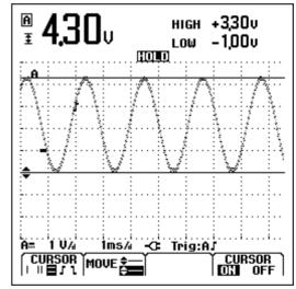
Figure 1-19. Voltage Measurement with Cursors
