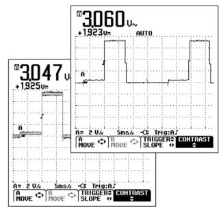
Figure 1-11. Smoothing the Waveform
