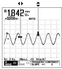
Figure 1-10. Positioning the Waveform
