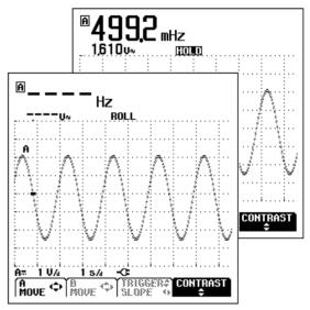
Figure 1-15. Recording Waveforms over Longer
