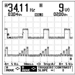
Figure 1-8. Hz and Vpp as Main Readings
