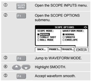
You can use waveform smooth to suppress noise without loss of bandwidth. Waveform samples with and without smoothing are shown in Figure 1-11.
