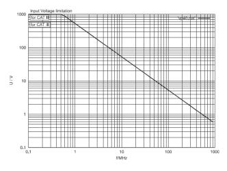
Figure 4-2. Max. Input Voltage v.s. Frequency for VP40 10:1 Voltage Probe
