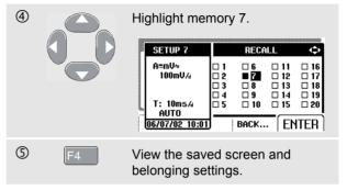
Observe that the recalled waveform is displayed and that HOLD appears on the screen. From this point you can use cursors for analysis or you can print the recalled screen. The instrument returns to signal acquisition if you press the HOLD/RUN key. The settings such as stored in memory location 7 are used then.
