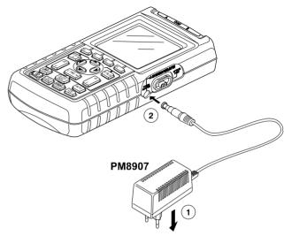
Figure 2-1. Charging the Battery Pack
