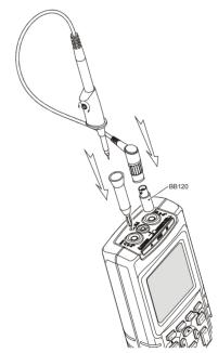
Figure 2-3. Adjusting Scope Probes
