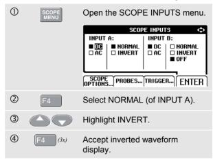
For example, a negative-going waveform is displayed as positive-going, providing a more meaningful viewing perspective in some cases. An inverted display is identified by trace identifier  $\triangle$  on left of the waveform area.
