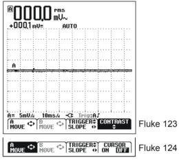
Figure 1-2. The Screen After Reset
