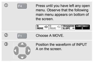
Waveform positioning is demonstrated in Figure 1-10.
