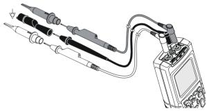
Figure 3-3. Grounding with Unshielded Ground Lead
