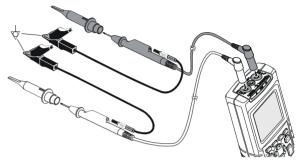
Figure 3-2. Grounding with Short Ground Lead
