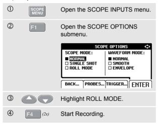
The waveform moves accross the screen from right to left like a normal chart recorder. Observe that during recording no measurements are made. (See Figure 1-15.)
