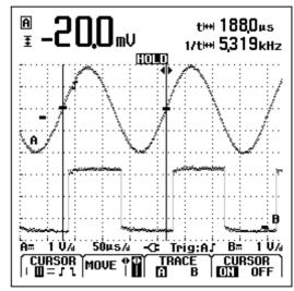
Figure 1-20. Time Measurement with Cursors
