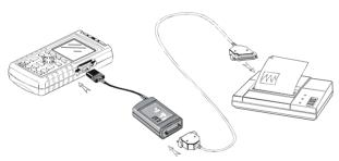
Figure 1-23. Connecting a Parallel Printer
