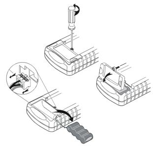
Figure 2-2. Replacing the Battery Pack
