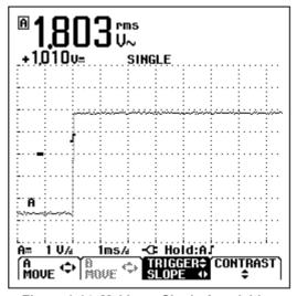
Figure 1-14. Making a Single Acquisition
