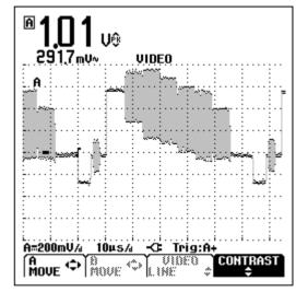
Figure 1-18. Measuring Video Signals
