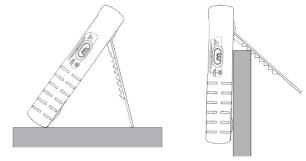
Figure 3-1. Using the Tilt Stand
