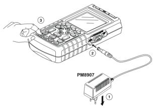
Figure 1-1. Powering the Test Tool
