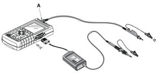
Figure 1-17. Isolated Triggering
