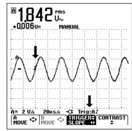
Figure 1-16. Screen with all Trigger Information
