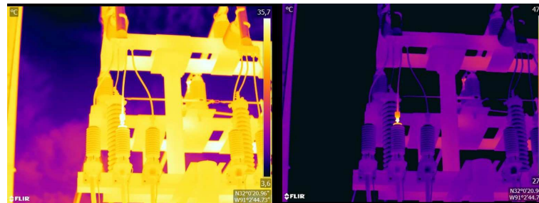
Figure 34.8 A thermal image in automatic mode (left) and in manual model (right). The adjusted temperature interval increases the contrast in the image and makes the faults clear.
