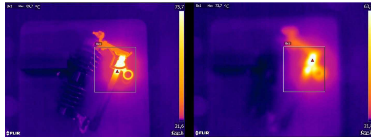
Figure 34.2 Focused thermal image (left) with a maximum temperature of T_{\max} = 89.7^{\circ}\text{C} ( 193.5^{\circ}\text{F} ) and an unfocused thermal image (right) with a maximum temperature of T_{\max} = 73.7^{\circ}\text{C} ( 164.7^{\circ}\text{F} ).
