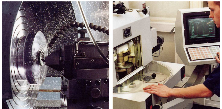
Figure 12.4 LEFT: Diamond turning machine; RIGHT: Lens polishing
