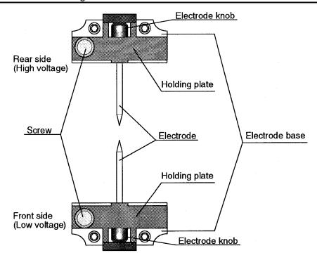
♦ When cleaning an electrode, grasp the electrode at its center to prevent it from bending and polish the tip with a knife sharpening block.
