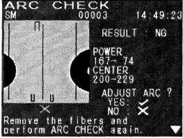
center pixel of the melt back by pressing ✓. When the measured center is out of the automatic correction range of 240+/- 40, "ARC ERROR" is displayed after the "RESULT: NG", and the screen instructs that the electrodes should be cleaned or replaced.
