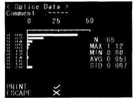
4. Press ✓ to print with the S902 printer or to output to a PC (personal computer). Printing or outputting the data will take some time according to the quantity of the data and the operating keys do not work during the time.
