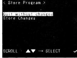
8. To store the changes, select "Store Changes" and press ✓. The screen changes to the location menu for the store. Storing the program at "CURRENT" stores the change on the current fusion program and the change disappears when the power is turned off. Storing at "BACKUP RAM" enables to store the modified program at a location from 32 fusion program locations except No. 1 to 3 where DEFAULT Programs are stored. It can be reinstalled for splice at the next power on.
