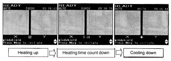
♦ To stop the heating operation (the HEAT LED is lit), press ❤. The heating stops and the cooling starts immediately. The cooling fan also stops by pressing ❖ again.
