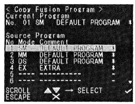
**4.** Using the  $\triangle$  or  $\nabla$ , highlight the location for the new program and press  $\checkmark$ .
