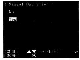
3. Use the keys indicated to manually operate the motors and perform the splice. If the distance is left at zero then the + / - keys can be used to operate the selected motor in **a** forward or reverse movement. The arc can be discharged when the highlight is not at "Move". The first arc arc is discharged with Cleaning Arc parameters, second with Fusion Arc parameters and with Additional Arc parameters thereafter.
