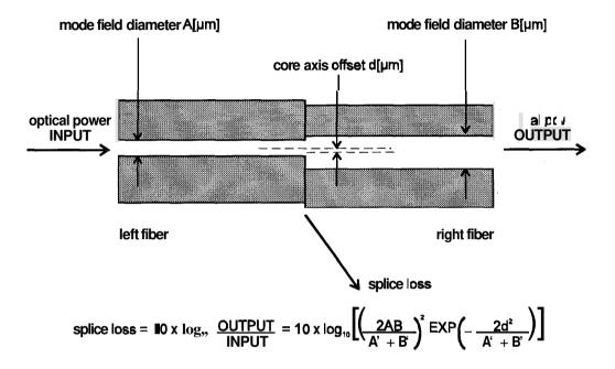
A difference between A and B will cause a splice loss, even if d is zero. If using single-mode fiber, the manufacturer of the fiber may be able to provide mode field diameter specifications.
