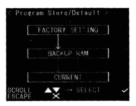
2. Using the  $\triangle$  or  $\nabla$ , scroll to highlight the program (machine, fusion, heater or all) where the default factory settings are to be sent, and press  $\checkmark$ .
