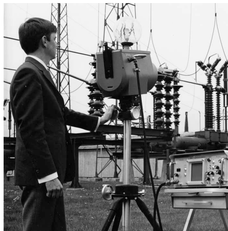
Figure 31.2 1969: Thermovision Model 661. The camera weighed approximately 25 kg (55 lb.), the oscilloscope 20 kg (44 lb.), and the tripod 15 kg (33 lb.). The operator also needed a 220 VAC generator set, and a 10 L (2.6 US gallon) jar with liquid nitrogen. To the left of the oscilloscope the Polaroid attachment (6 kg (13 lb.)) can be seen.
