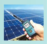
Extech's SP505 measures solar power level from outdoor sunlight to determine the best location of solar panel and solar water heater installations. It is also used indoors by window manufacturers, automotive industry, and remodeling home owners to check the level of solar radiation transmission through various glass thicknesses and degrees of tinting to use for window installations. Convenient pocket-sized meter with built-in precision solar light sensor is easy-to-use wherever you go.
