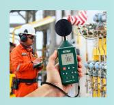
Extech's ultra-compact sound meter meets class 2 standards with ±1dB high accuracy that allows for quick and reliable sound level testing. It features a large backlit display for easy viewing and measures A & C weighting from 35 to 130dB with Fast and Slow response time mode. Size is small enough to conveniently fit in your pocket and includes a wrist strap.
