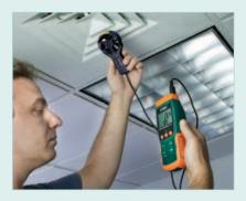
Typical application of measuring air velocity and temperature in HVAC
