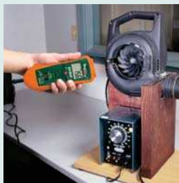
Non-contact model for use on machinery where high speed measurements are required
