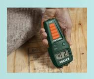
Take quick moisture level reference measurements on wood and building materials with this convenient compact-sized pin-type Moisture Meter. Easy-to-operate with display icons that indicate the levels of moisture content plus audible alert feature. Ideal for building restoration projects and applications where moisture detection on floors and under carpets is critical. A must-have tool for analyzing the after-effects of water leakage behind walls and in ceilings.
