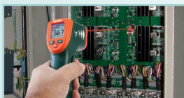
Detect hot spots on circuit breaker panels
