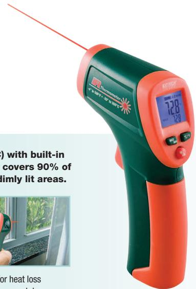
**Compact non-contact InfraRed Thermometer measures up to 500°F (260°C) with built-in laser pointer to identify target area and improve aim. Fixed 0.95 emissivity covers 90% of surface applications. Backlighting for taking measurements at night or in dimly lit areas.**
