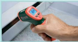
Test for temperature in heating systems
