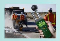
Extech's Heat Stress WBGT (Wet Bulb Globe Temperature) Meter accurately determines the Heat Stress level (how hot it feels outside) by factoring a combination of humidity, temperature, air movement, and direct solar radiation. These factors all affect how hot our bodies get, as well as our ability to cool down. It's perfect for monitoring the Heat Index on hot humid days to prevent heat stroke during road or building construction, outdoor activities, sporting events, or in the workplace.
