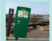
Compact handheld Conductivity Meter with long life carbon rod combination electrode measures Conductivity, TDS and Temperature. Units of measure include  $\mu$ S/cm, mS/ cm, ppm, °F, and °C. The meter features three ranges for Conductivity and TDS plus adjustable Temperature compensation factor to maintain accuracy.
