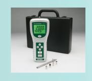
Push/Pull measurements in oz, g and Newton (475040-SD) or lbs, kg, and Newtons (475044-SD) units on dual LCD with reversable display feature to match viewing angle. Ideal for a wide variety of applications in the electronics, automotive, chemical, plastics and machinery industries.
