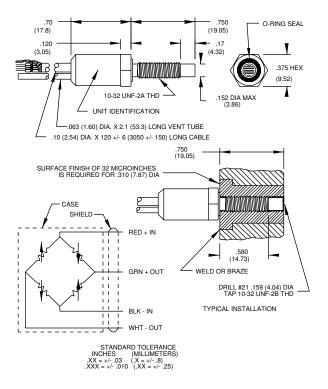
ENDEVCO Model 136 Three-Channel System, Model 4428A or 4430A Signal Conditioner, or OASIS 2000 Computer-Controlled System are recommended as signal conditioner and power supply.
