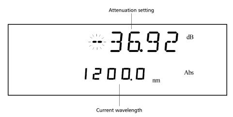
**2.** Enter a new attenuation value. Use the up/down arrows to change the flashing digit and the left/right arrows to activate the next digit.
