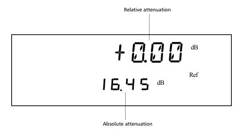
If the attenuation is increased by 1.0 dB, the upper digits (relative attenuation) will display **-1.00 dB** and the lower digits (absolute attenuation) will indicate **-17.45 dB**.
