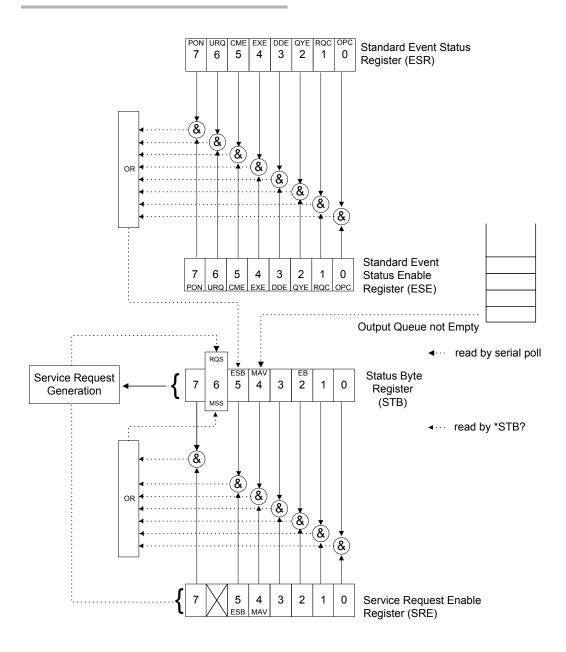
An SRQ is forced when a bit is set in the STB and at the same time the corresponding SRE bit is set. When the SRQ is generated, the RQS bit is set to 1 and remains set until read by a serial poll. Once the RQS is read, it returns to 0.
