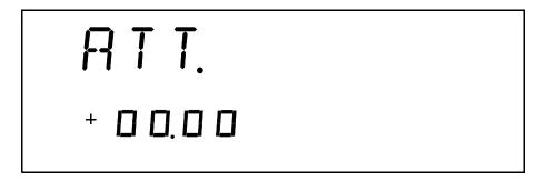
**12.** Press ENTER. The first segment will start flashing. Use the up/down arrows to change the flashing digit and the left/right arrows to activate the next digit.
