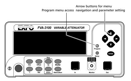
**2.** Press ENTER. The first digit will start flashing. Use the up/down arrows to change the flashing digit and the left/right arrows to activate the next digit.
