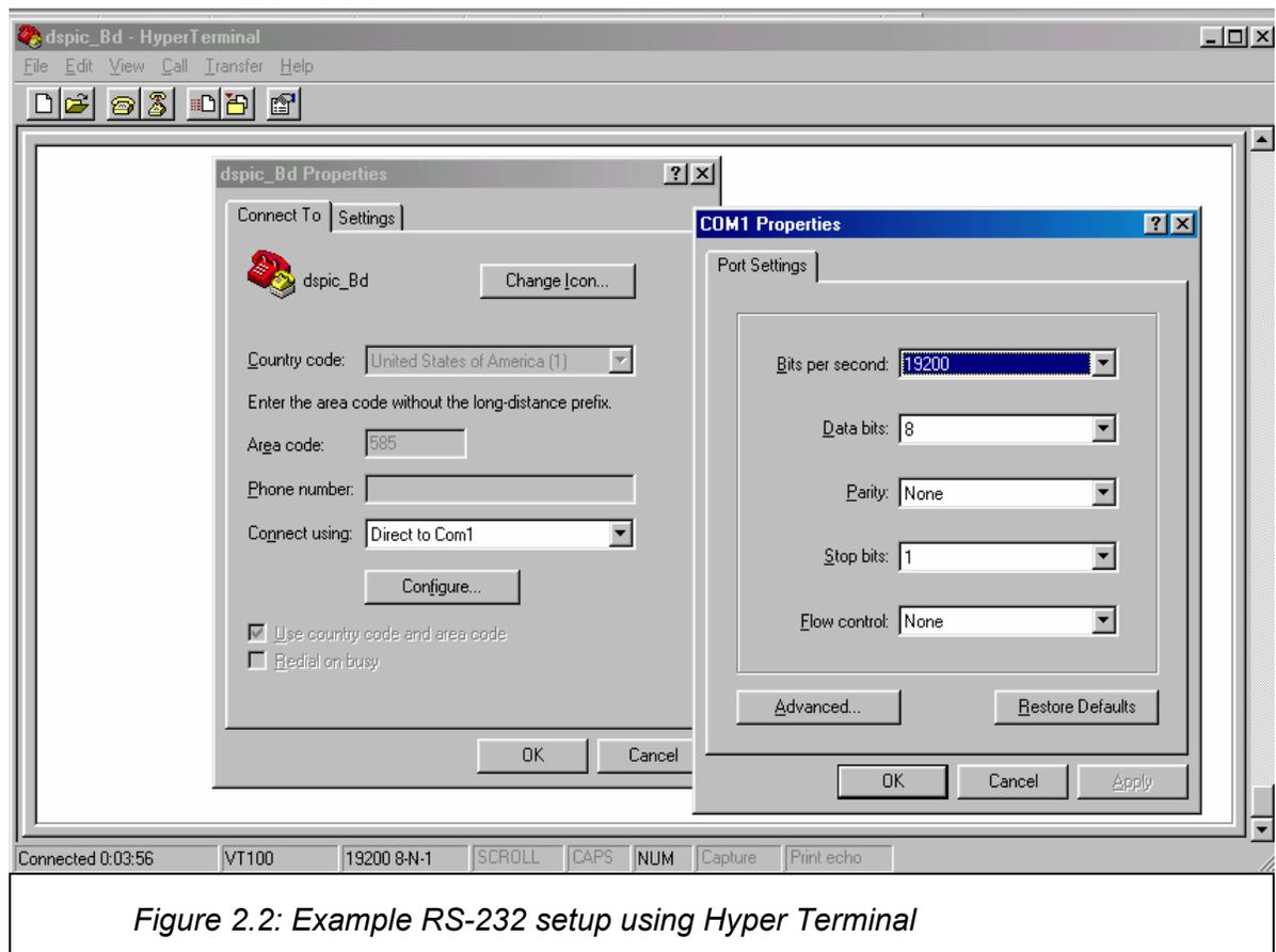
Figure 2.2: Example RS-232 setup using Hyper Terminal
