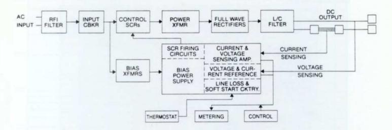
In an SCR phase-controlled DC Power Supply, output is controlled by modulating the conduction angle of the controlling SCRs. The EMHP Series, input AC is applied to pairs of bi-directionally connected SCRs placed within the primary circuit of the main power transformer. The secondary voltage of this transformer is rectified and L/C filtered to provide a low ripple DC output. Both output voltage and
