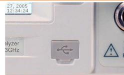
The USB icon turns On when the flash drive is detected.
