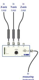
The loops are constructed from high quality RG 223/U coaxial cable, inside flexible 1" PEX pipe. The three (3) loops connect to three (3) current to voltage transducers, the outputs of which connect to three respective inputs on a coaxial switch.
