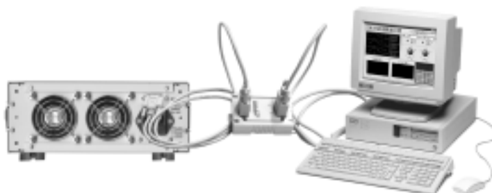
Fig.1-1 Connect the electronic load to PC
