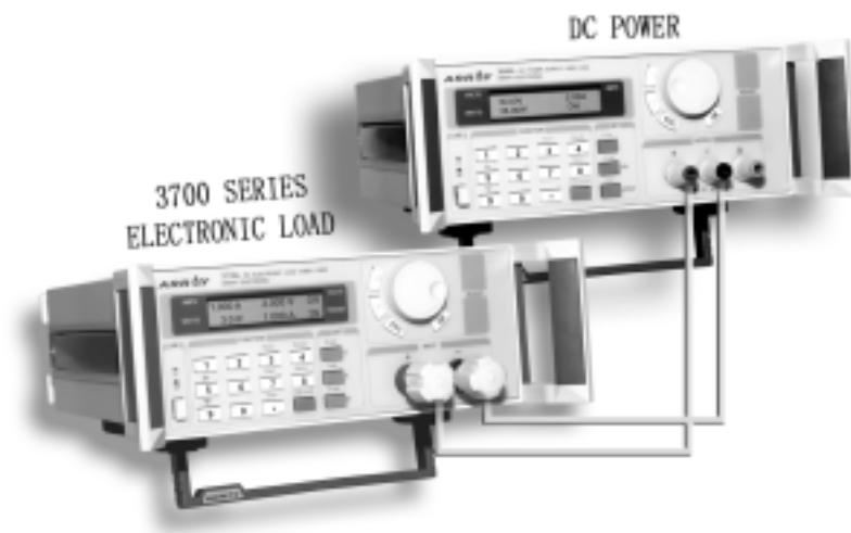
Fig.2-1 Connect the power supply to the electronic load
