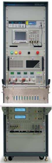
DC to DC Converter ATS
