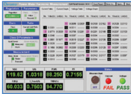
IEC 61000-3-2 Current Harmonic Test
