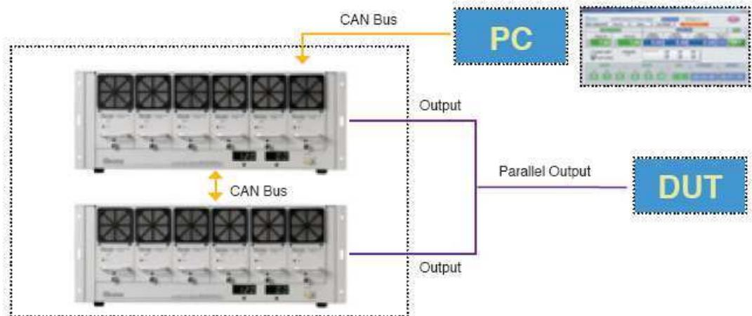
**Type C - Control without CSU or PC :** User can only control via remote on/off signal for paralleled operation.
