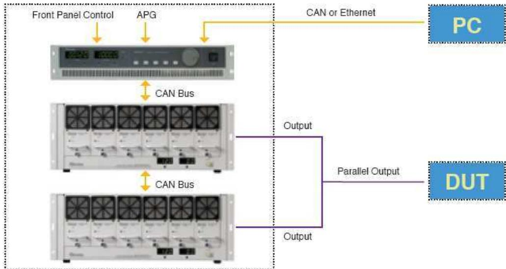
**Type B - Control without CSU :** User can only control via CAN Bus for paralleled operation.
