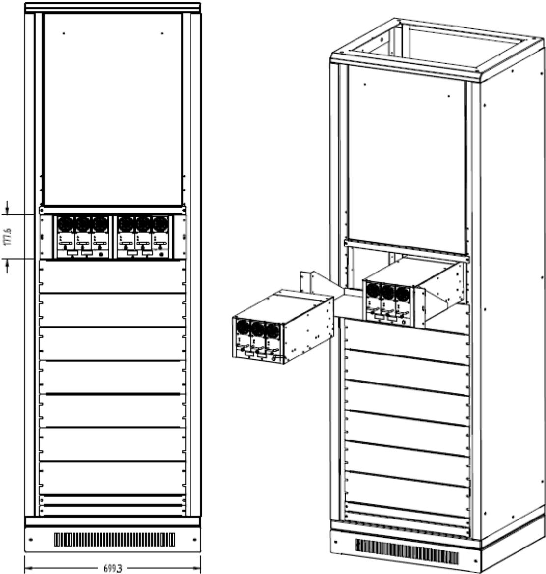
For 23" rack each 4U can assemble 2 sets of 62000B-3-1
