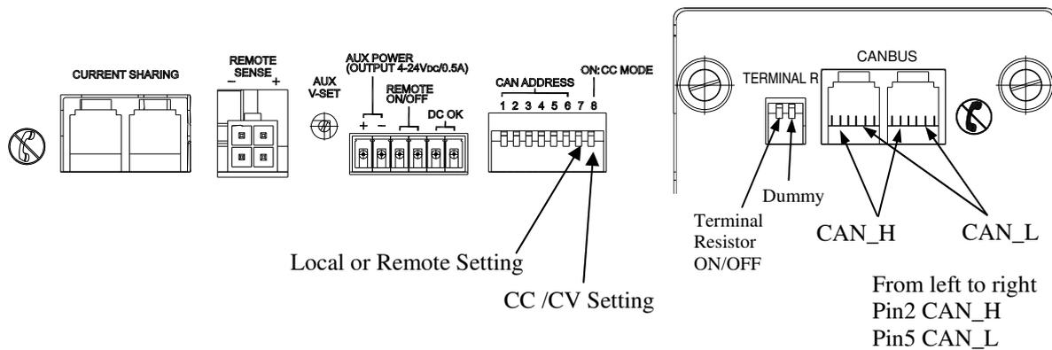
Figure 1-5 Communication Contacts on the Rear Panel
