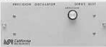
The model 855T is designed for those applications where access to the frequency adjustment is to be limited. Frequency changes are by means of an internal DIP switch which can be set from 45Hz to 9999Hz. Amplitude adjustments are by a front panel control (optional "locked" amplitude control is available).
