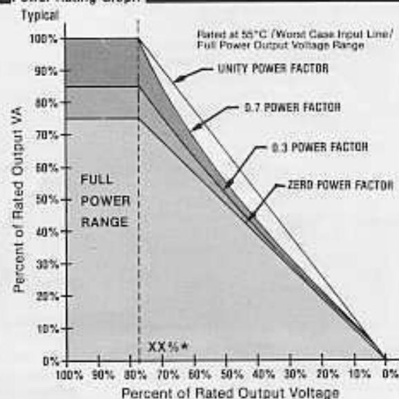
\* Unique to California Instruments is the "range rated" full power capability. All California Instruments T Series power amplifiers are capable of delivering full power from XX% to 100% of rated output voltages. For most power amplifiers, this full power range is from 78% to 100% of rated output voltages.
