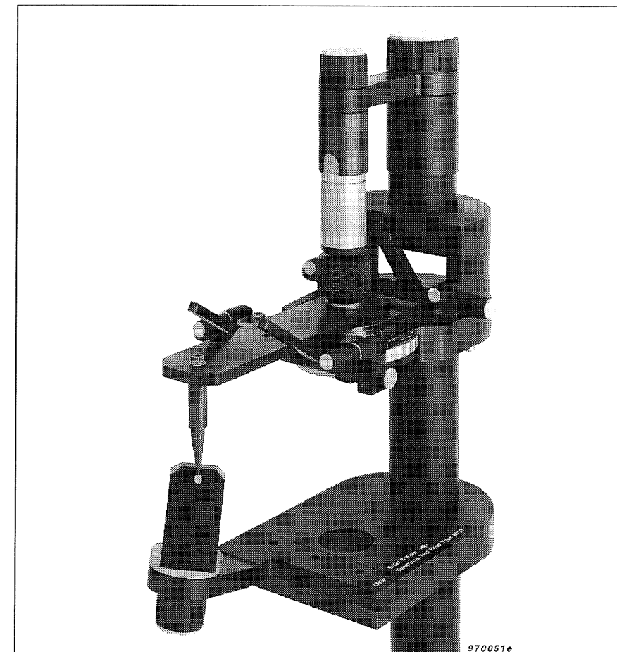
Fig. 2.9 Telephone Test Head fitted with test templates for checking the LRGP and AEN speaking positions
