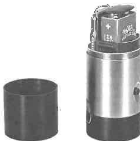
Fig.2.3. 9 V Battery Installed in the Calibrator
