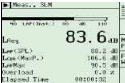
Fig. 8 Multi-D screen showing real-time simultaneous display of broadband parameters and Elapsed Time
