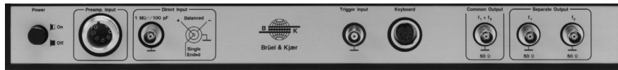
Fig. 14 Input/output panel of the 2012, showing the 7-pin Preamplifier Input for connection of Brüel & Kjær condenser microphones, and the Direct Input which can be single ended or differential (balanced)
