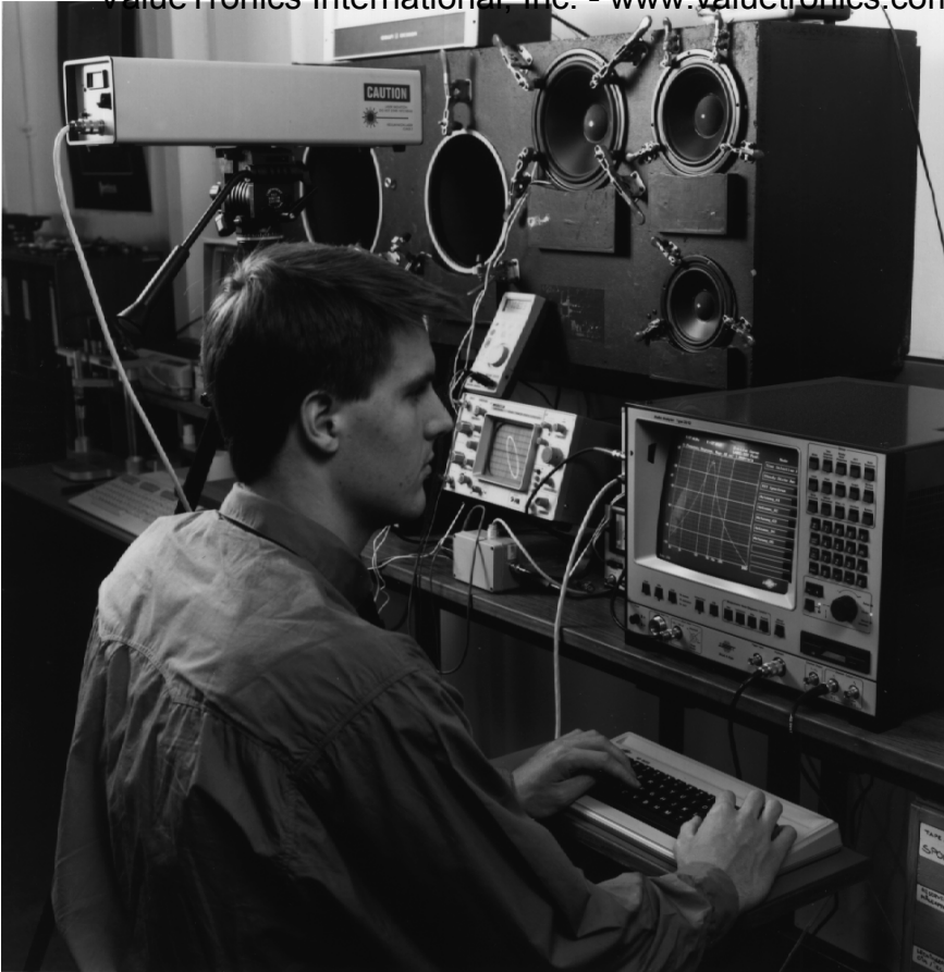
Fig.15 Type 2012 is ideal for transducer measurements. The setup in the picture uses the Laser Transducer Set Type 3544 for measuring the Thiele-Small parameters. Use of the laser enables measurements without the mass-loading effects of an accelerometer
