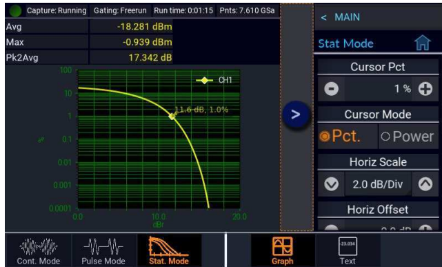
Figure 3-8. CCDF Plot With Menu Showing Cursor at 1%
