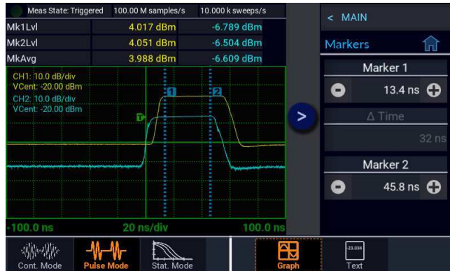
Figure 3-6. Marker Measurements on CH1 and CH2 Pulses
