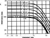
Accuracy: at 100 mV test level
