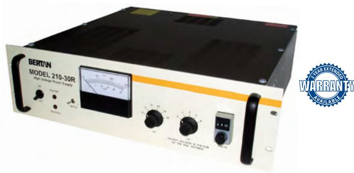
Spellman's Bertan brand of 210 Series of 125 to 225W high voltage power supplies provide regulated high voltage outputs from 1 to 50kV. The low noise, linear topology employed results in extremely low output ripple specifications. Units are inherently reversible by design, providing either positive or negative output polarity. The 210 is fully arc and short circuit protected. Excellent regulation specifications are featured along with outstanding stability performance.
