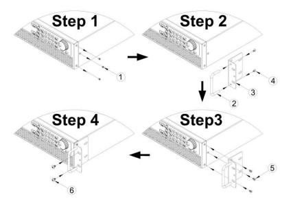
Figure 2.3 - Rack Mount Bracket Assembly
