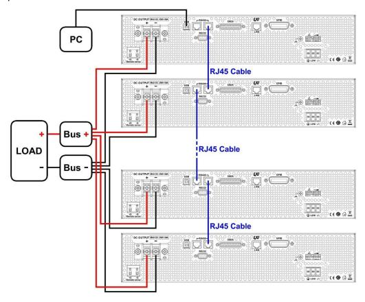
Figure 4.1 - RS485 Connection Diagram for 10+ Units
