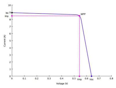
Figure 3.11 - PV Simulation Curve
