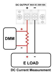
Figure 5.2 - Current Calibration Diagram
