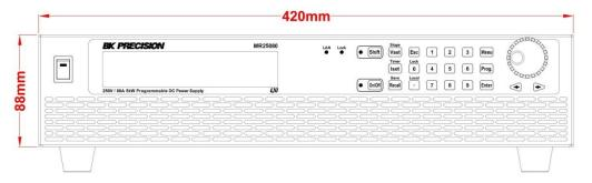
Figure 1.1 - Front Panel Dimensions
