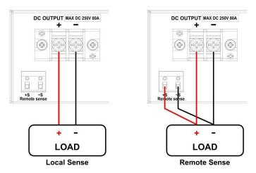
Figure 3.1 - Local/Remote Sense Connection Diagram
