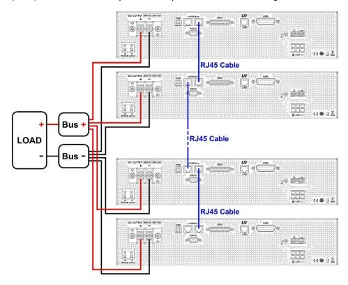
Figure 3.10 - Parallel Connection Diagram
