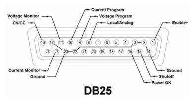
Figure 3.3 - DB25 Pinout
