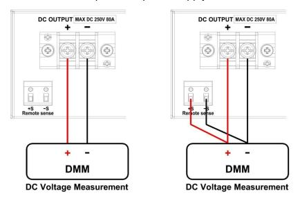
Figure 5.1 - Voltage Calibration Diagram
