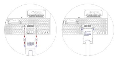
Figure 2.1 - AC Power Connection Diagram
